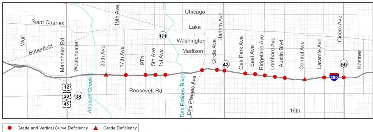
Figure 1-14 - Existing Crossroad Vertical Geometry Deficiencies
